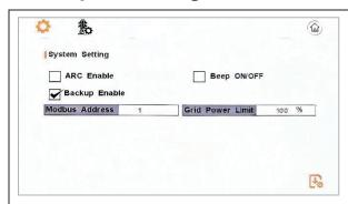
**ARC Enable**: ARC detection function. **Beep ON/OFF:** Screen alarm switch. Set enabled, the buzzer will sound when the inverter alarms.
