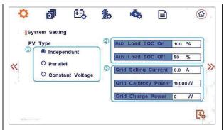
① Users can set PV types, including Independent, Parallel and Constant Voltage. ② load2 Enable or disable the value. If the Battery SOC is less than the set Off value, load2 shuts down. If the Battery SOC is greater than the set on value,
