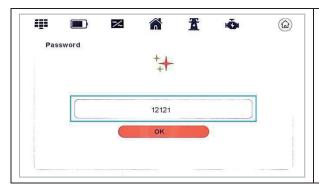
To enter the Maintenance settings, a password is required. The default password is 12121. Click OK to enter the settings interface.
