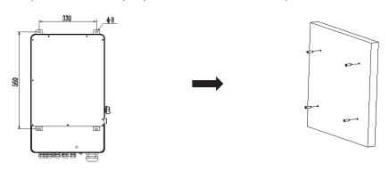
**Step 2**: Lift the inverter and align the hole of the inverter with the expansion bolt, Fix the inverter on the wall.
