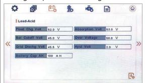
Float Chg Volt: Charge the battery with constant voltage and small current (This interface is used to set the lead acid battery charging voltage. (The input value ranges from 40 to 59.5) Set the floating charge voltage to be less than the constant charge voltage).
