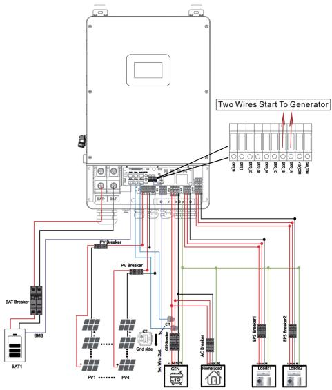
2) The Generator is normally connected to the Generator port. The connecting cable between the Generator and the inverter does not need to be covered with CT. The connection line of the power grid port should be connected with CT. The system diagram is as follows.
