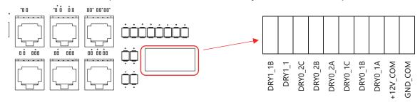
DRY1 1B/DRY1 1: Used to start the driver.
