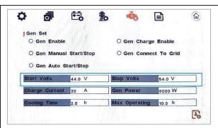
**Start Volt:** Generator in automatic mode. When the volt of battery is lower than the setpoint, the Generator dry contact is turn-on and the connected Generator will be started.
