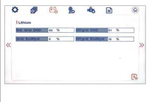
Bat Grid DOD/ Off-grid DOD: When the battery discharge is higher than the set parameter, the inverter generates a battery low voltage alarm. Distinguish between grid-connected alarm parameters and off-grid alarm parameters.
