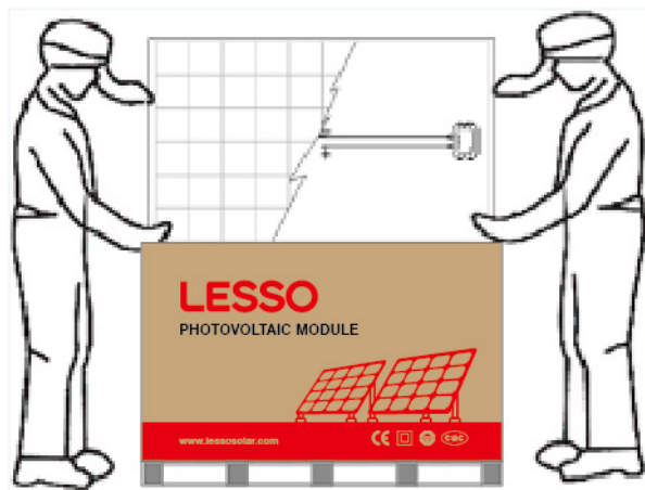
Figure 2 - Removing PV modules from a pallet
